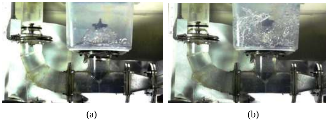
Figure 6. View of the valves position: (a) the waste valve full opened and the delivery valve full closed, (b) the waste valve full closed and the delivery valve full opened
