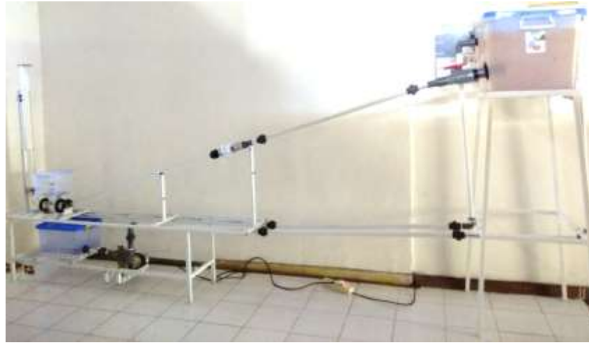
Figure 3. Experimental arrangement of the hydraulic ram
