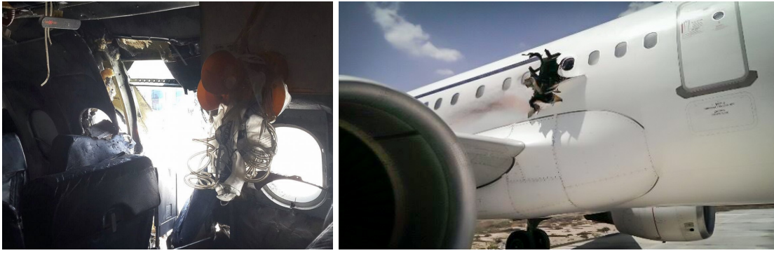
Figure 3.1: February 2016, Daallo Airlines: the one meter sized hole caused by an internal explosion.
