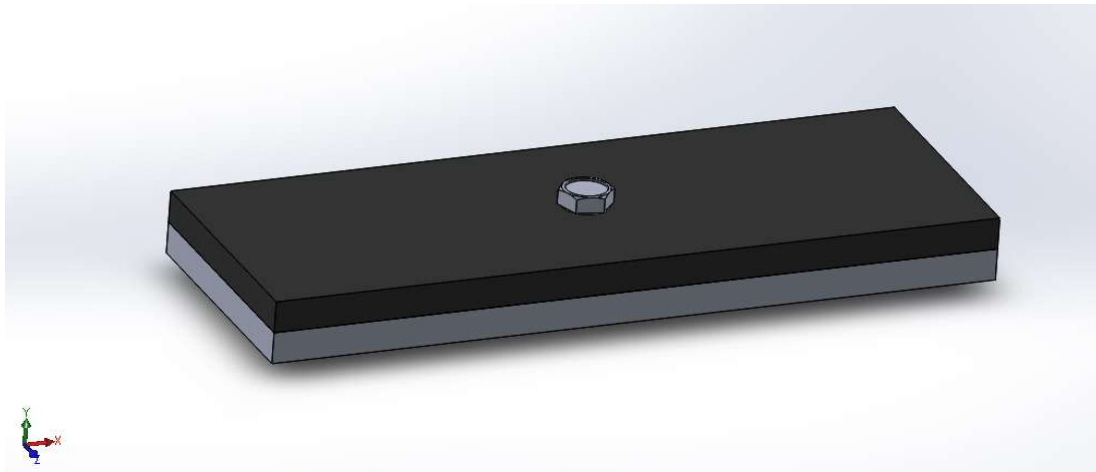
Figure 13 Grey Cast Iron- Aluminium Alloy 1060-H12 joint, 10 mm hole diameter for bolt entrance
