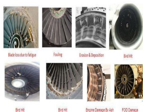
Figure 8 Types of Gas Turbine Faults
