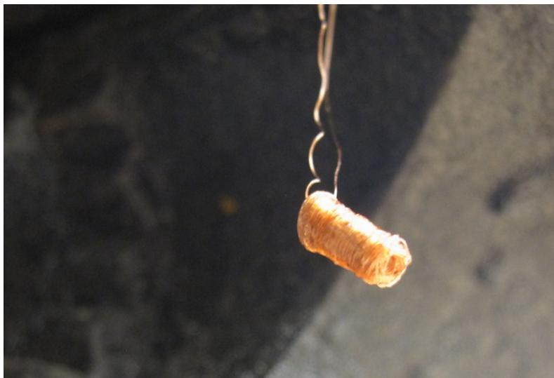
Figure 4.: Photograph of a 44 gauge wire coil used to test heat dissipation.
