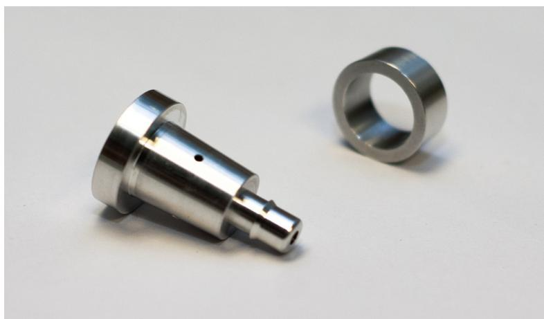
Figure 16.: Machined prototype of the second valve design.
