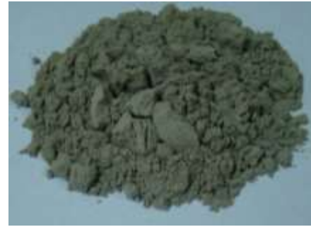
Ground Granulated Blast Furnance Slag(GGBS)
