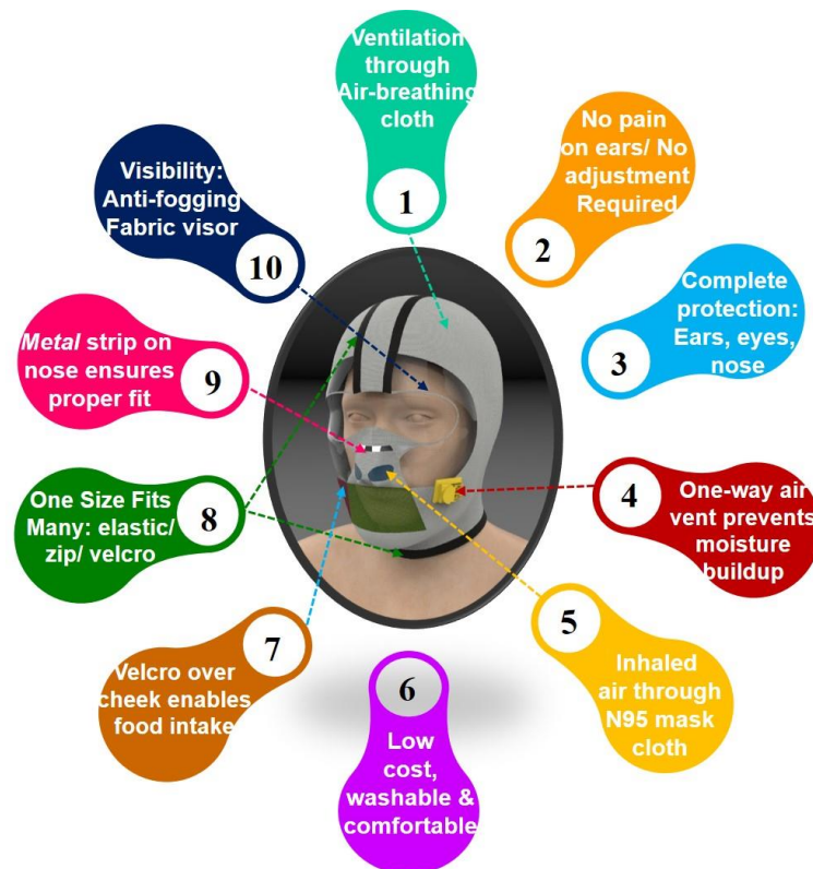
Figure 2: A schematic of the different features of fabric-helmet.
