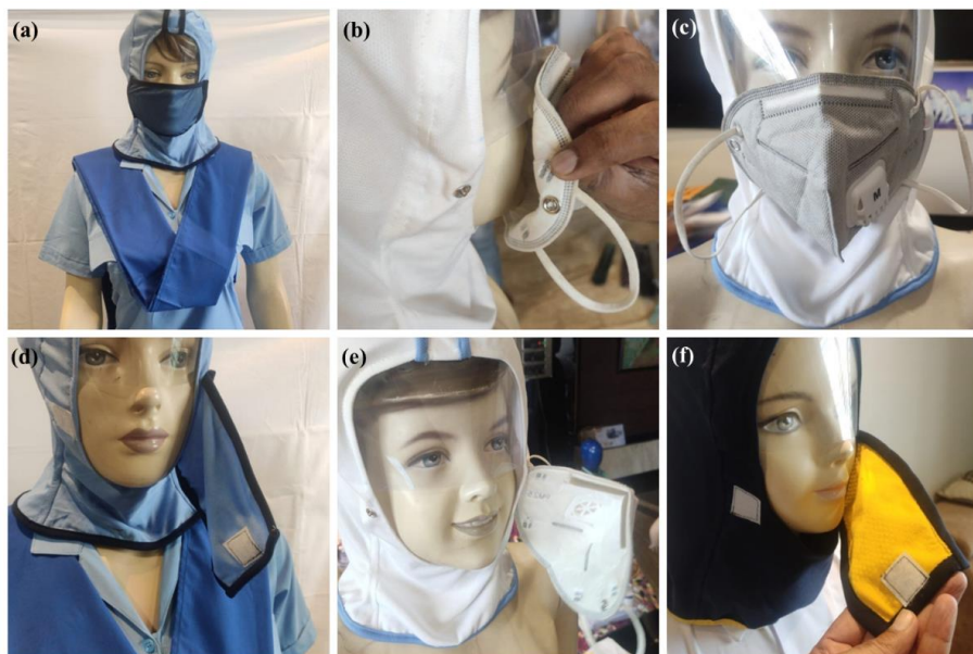
Figure 7: Mannequin models wearing different prototype designs of COVID fabric helmets designed for school children during testing phase: (a) Design-1 with mask closed, (b) Design-2 showing chit-button for masks, (c) Design-2 with N-95 mask, (d) Design-1 with mask open, (e) Design-2 with mask open, and (f) Design-3 with mask open, meant for small children.
