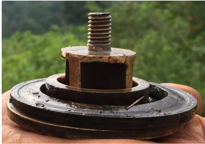
Fig 3A: Original check valve
