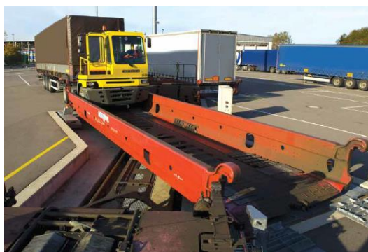
Figure 6. Example of intermodal trailer with horizontal loading, the “Modalohr” system currently used in the analysed section of the Mediterranean corridor.
