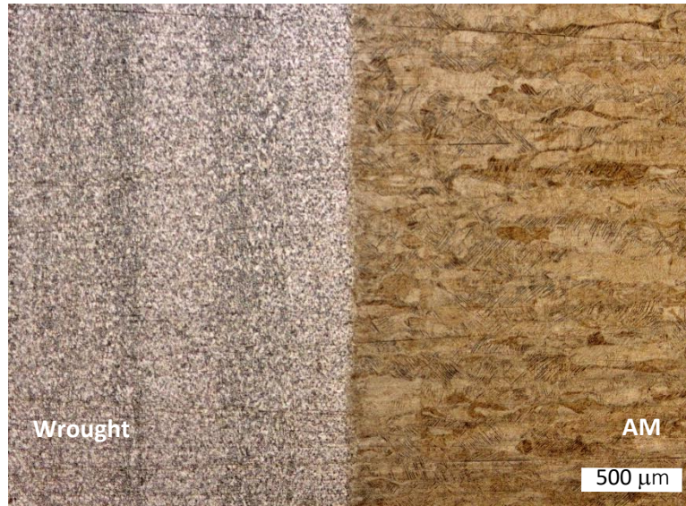
Figure 3: Optical microscopy image of the AM-wrought interface taken at a magnification of 5X
