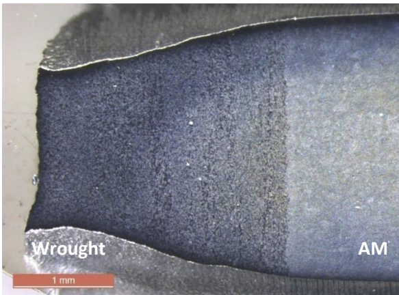
Figure 11: Typical tensile hybrid specimens post-failure. The specimens were ground, polished, and etched to aid in visualizing the location of the interface. Note that necking and failure have occurred in the wrought side and more than 1mm away from the wrought/AM interface.
