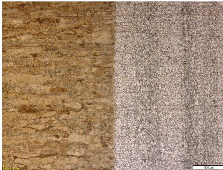
Figure 4: Optical microscopy image of the AM (left)-wrought (right) interface taken at a magnification of 5X
