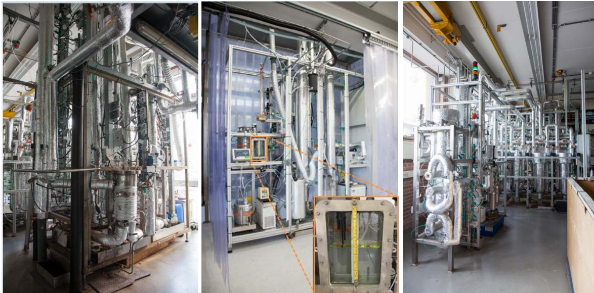
Figure 4 Picture of OLGA (left), BTX scrubber (middle), HDS unit and fixed bed reactors for sulphur removal (right).
