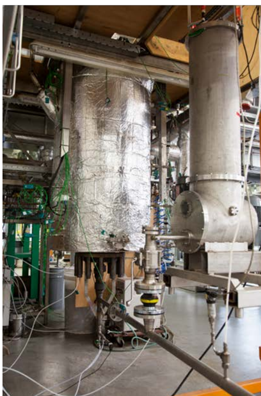
Figure 2. Picture and schematic layout of the 25 kW i-MILENA gasifier as used for lignin and beech wood gasification.
