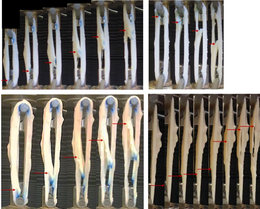
Figure S3: Images of mode II crack propagation in 4 samples undergoing the SFRT. Red arrows approximately indicate the position of the crack tip. Fibrils formed during fibrillation are observed in the top left pane of images.
