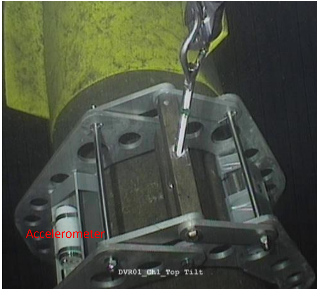
Figure 2 Clamp develop by DOF with accelerometer clamped onto a partially strake-covered span
