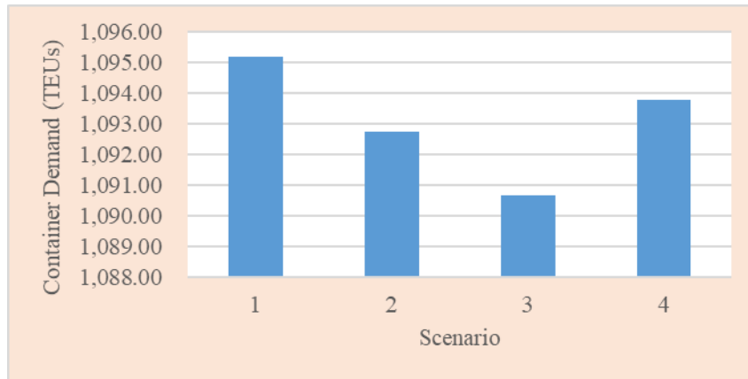
Figure 105 Sensitivity of the average container demand at ports to the availability of TWs.
