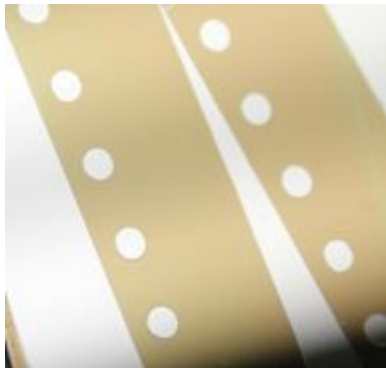
Figure 7. A silicon sample patterned using the benchtop Photolithography tool
