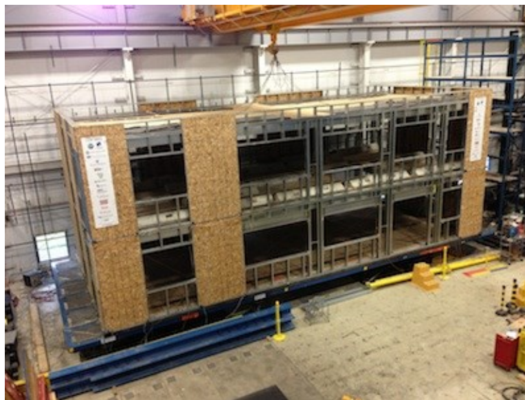
Figure 30. CFS-NEES test building on shake tables at University of Buffalo SEES Lab
