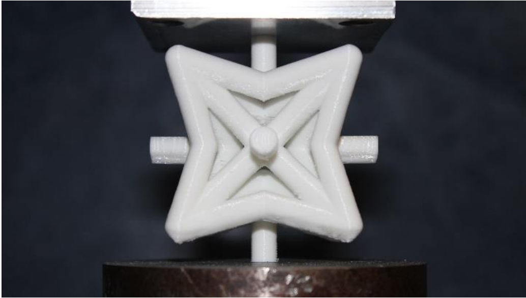
Figure 8: Test sample with \mu = 0.25 under compression testing
