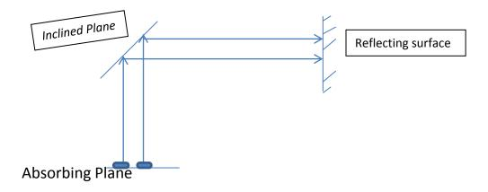
The idea is to plant lasers on one surface which is ideally made of an ideal Laser absorber. Lasers are fired normal to this surface producing force  $F_1$  on surface (actually, space craft) as shown in diagram 1. The lasers are reflected by ideally reflecting inclined plane, which produces a force  $F_2$  on inclined plane, normal to it. The lasers then fall on third surface, which is again a perfect reflector. This
