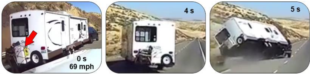
Figure 3 – Video snapshots of fishtailing event of a badly loaded caravan.
