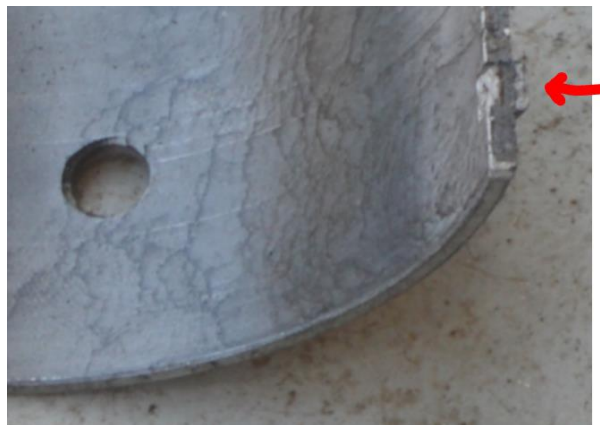
Figure 15 – Locating lug (red arrow)
