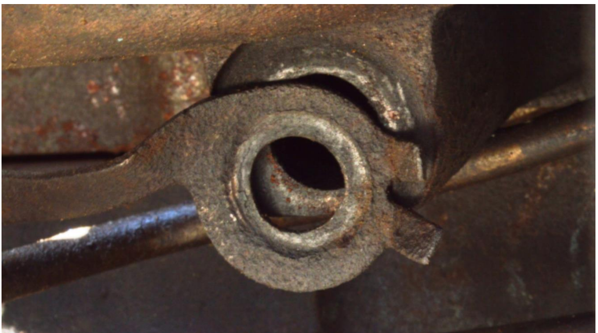
Figure 11 – Exhaust manifold stud missing
