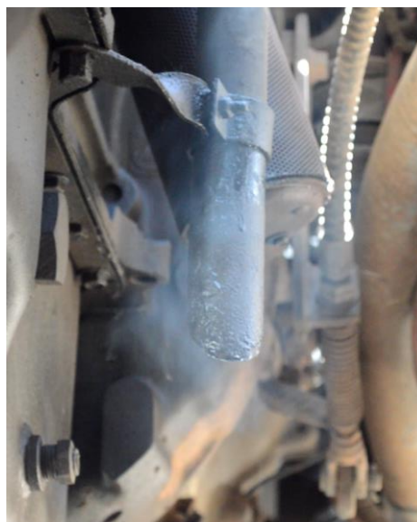
Figure 6 – Breather pipe emissions showing white smoke.
