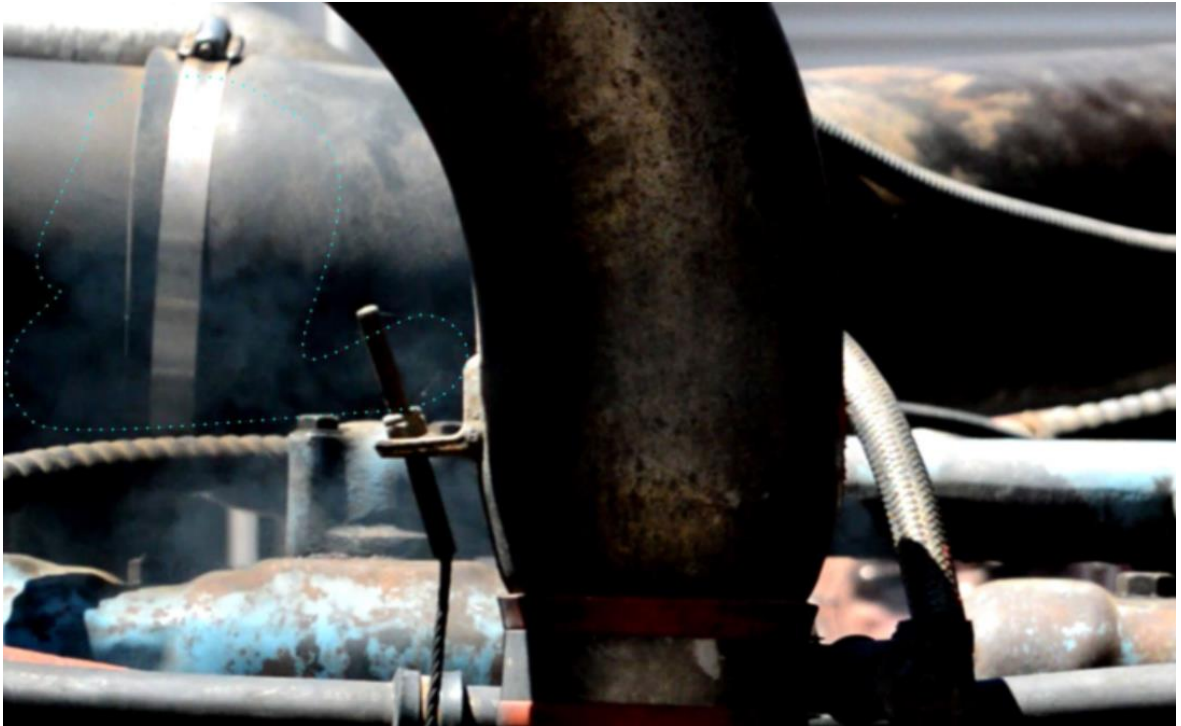
Figure 10 – Exhaust manifold leakage showing white smoke emission. (Screen capture of movie taken by the author from kerb-side) (Dotted outline of smoke by author)
