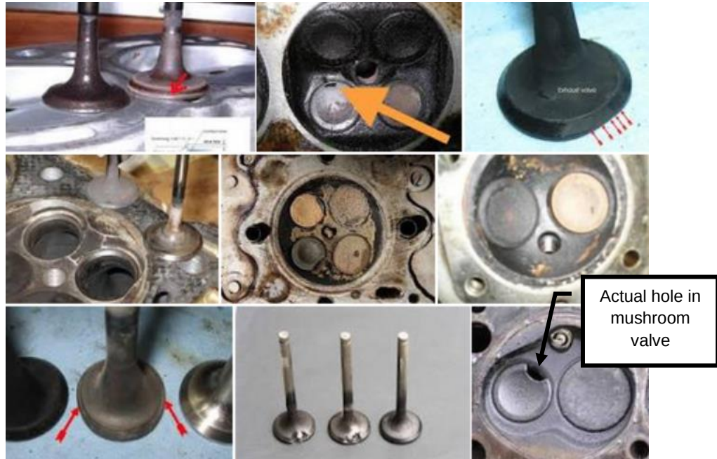
Figure 30 – Google search for “images of burnt valves”
