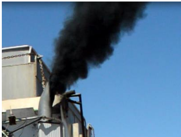
Figure 5 – Thick black plume of exhaust smoke during start and acceleration.
