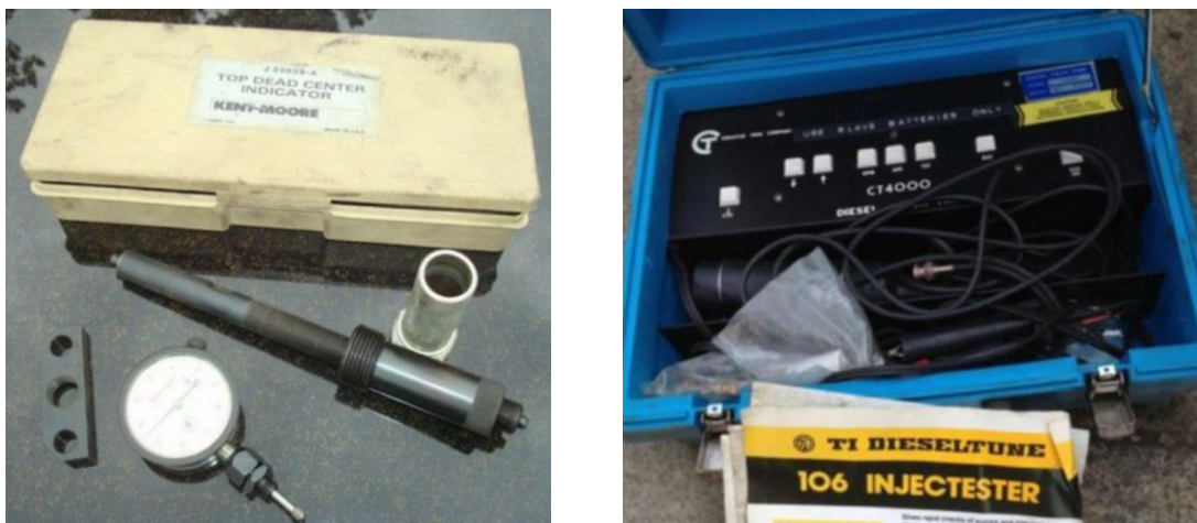
Figure 27 – Top Dead Centre Indicator and CT4000 Diesel Tach-Time
