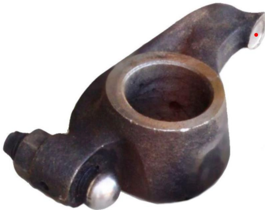
Figure 7 – Examination of a rocker arm highlighting wear by red dot.
