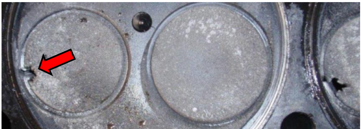
Figure 17 - Close-ups of burnt exhaust valves.
