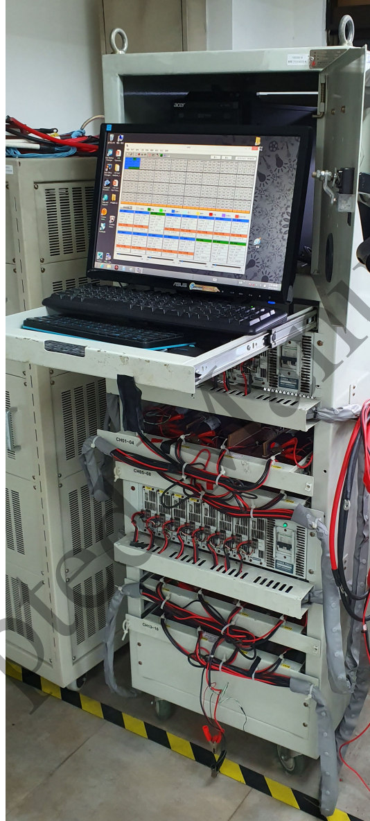
Figure 3. Battery test system. The CTE-MCP-5082020A battery test system (made by Chen Tech Electric Mfg. Co., Ltd., Taiwan) is used for evaluating the performance of the battery cells. There are 16 channels, and each of them can provide measurements of voltage, current, and temperature simultaneously.
