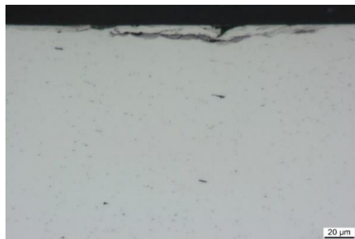
Figure 7: Exemplary figure of a material overlap due to rotary swaging. 1.4404, section III, unetched
