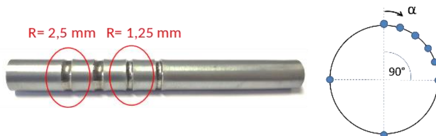
Figure 8: Position of the X-Ray residual stress measurements on the samples produced by recess rotary swaging
