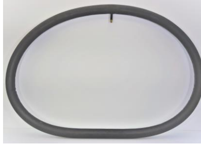
Figure 5 – Bicycle inner tube demonstrating geometric stiffness.
