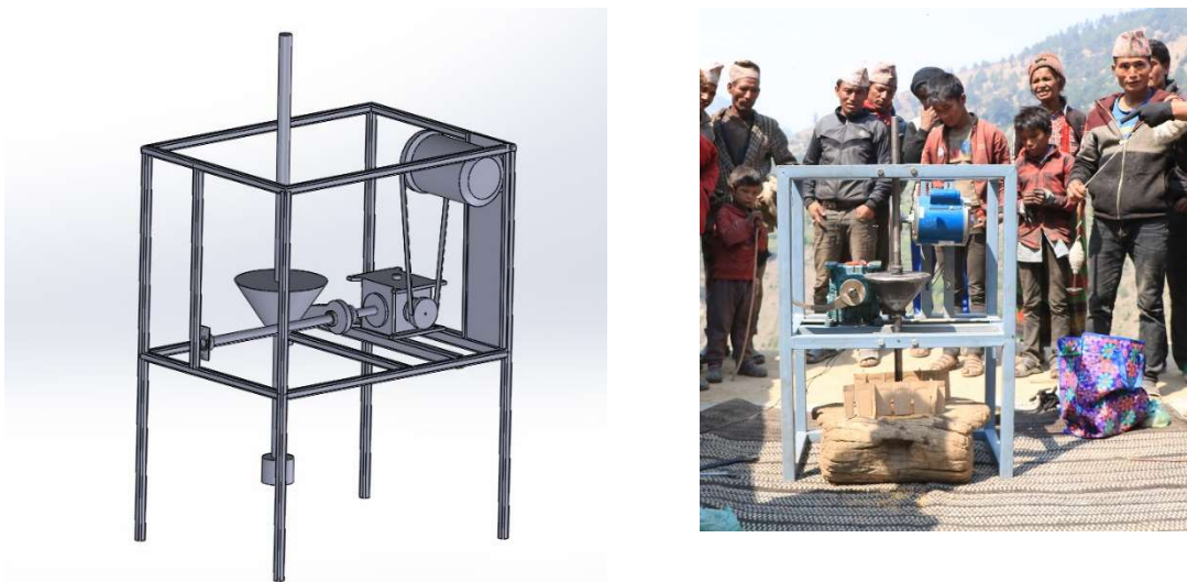
Figure 4 a. 3D model of the Prototype De-husking machine b. fabricated model of a.
