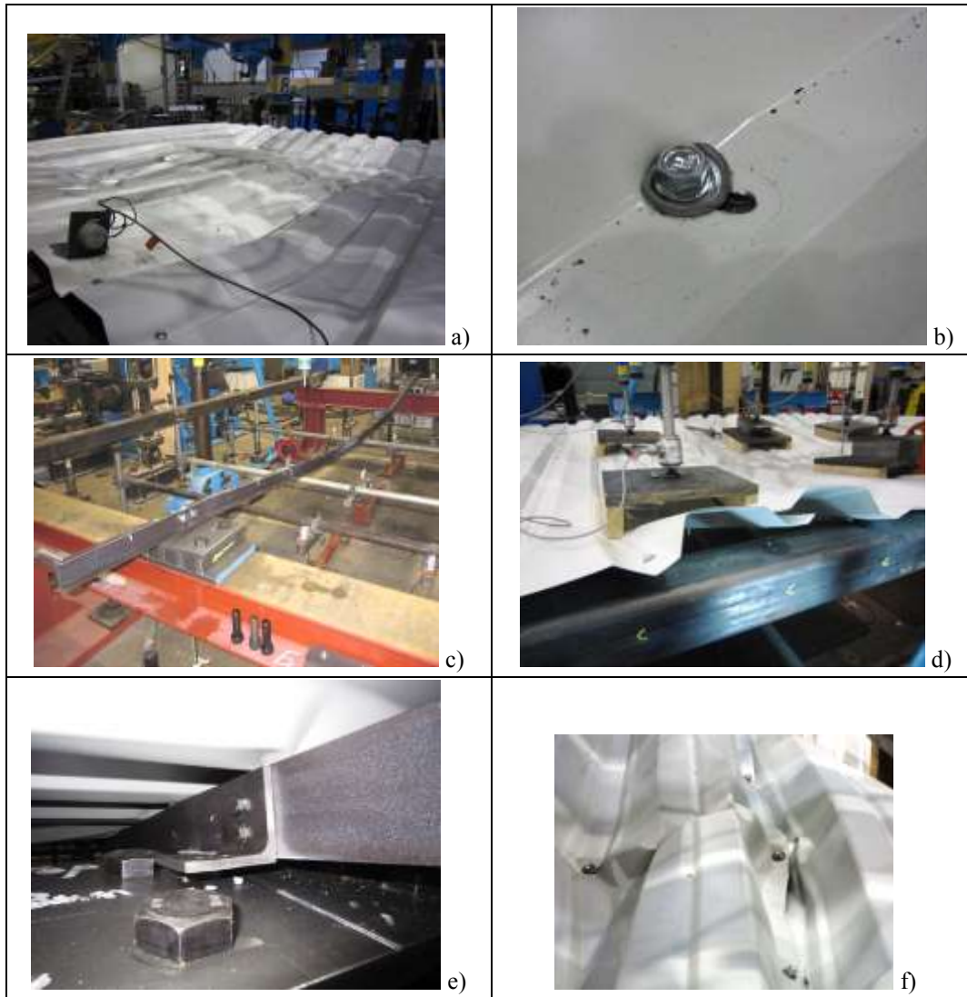
Fig. 3. Damage state at the end of tests a) residual deformations in B-TR35-100; b) bearing failure in B-TR35-100; c) plastic deformations in mid-purlin of Specimen D-TR35-100; d) screw failures in C-TR35-100; e) tension failure of bolts in purlin-to-column connection in E-TR35-100; f) localised deformations in H-TR84-075
