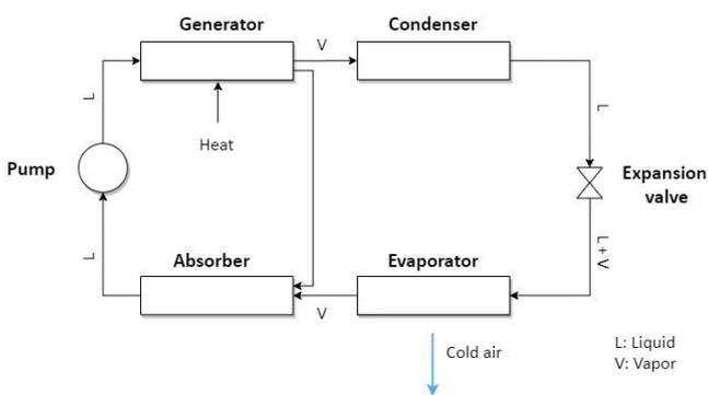
Figure 4 – Simple absorption process.
