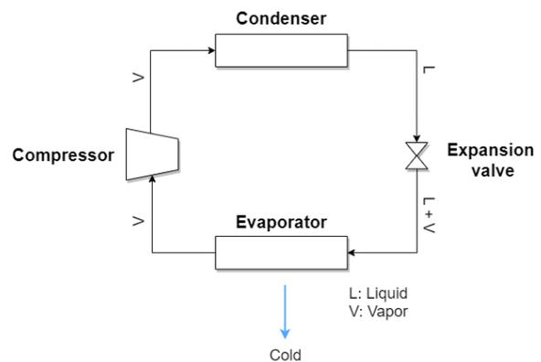
*Figure 2 - Vapour Compression Refrigeration process.*
