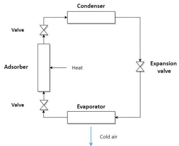
Figure 5 – Simple adsorption process.
