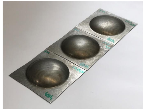
Figure 7: Results from the optically measured shapes of the formed pieces as a function of process parameters. A successive increase of process force shows the geometrical definition of the part in the rubber pad forming process. While the apex of the dome was reached after 100 kN, larger forces are required to calibrate the radius of the dome-shaped part.
