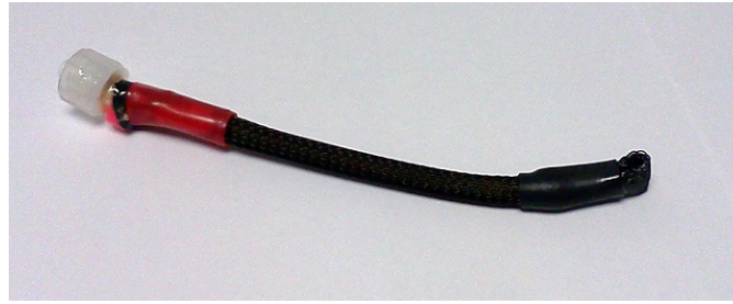
Figure 12. Photograph of a prototype artificial muscle actuator.
