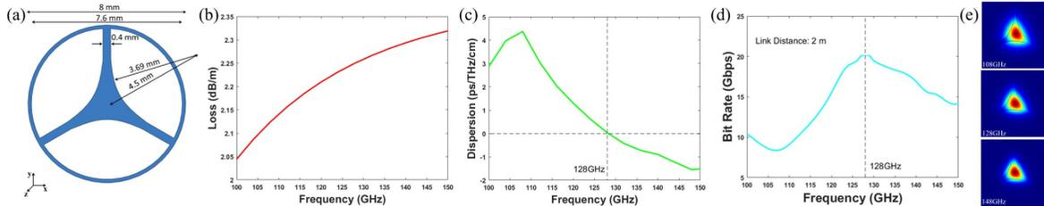
Fig. 1. (a) Schematic of the fiber cross-section, (b) modal losses, (c) dispersion, (d) bit rate and (e) normalized electric field distribution of the fundamental mode as a function of operation frequency near 128 GHz carrier.
