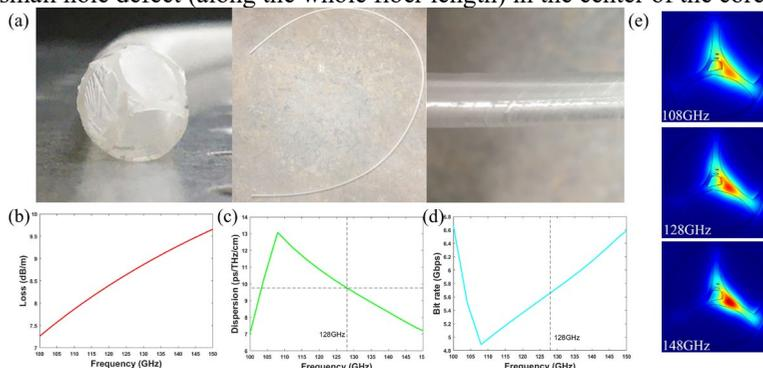
Fig. 2. (a) The cross-section, top view and side view of the fabricated fiber using an infinite 3D printer. The (b) loss, (c) dispersion, (d) bit rate and (e) normalized electric field distribution of the fundamental mode as a function of the operation frequency.
