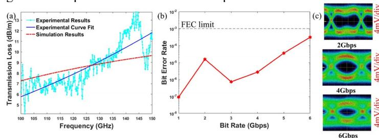
Fig. 3. Experimental characterization of the 3D printed fiber. (a) Transmission loss vs frequency, (b) Bit Error Rate vs Bit Rate and (c) measured eye patterns for different bit rates for a 0.75 m-long fiber.
