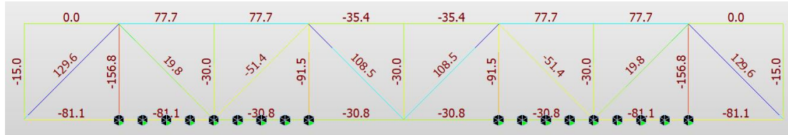
Fig.14 Internal force diagram of truss during jacking operation for multi-points support simulated surface support (unit: kN, negative value represents compression)
