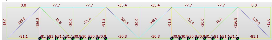
Fig.17 Internal force of truss with multi-point support (unit: kN, negative value represents compression)
