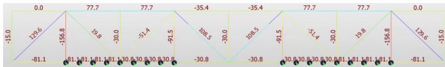
(a) Truss with multi-point support
