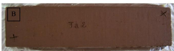
Figure 1: (A) Device for producing test specimens by the proposed method. (B) Example of a test specimen with the two reference crosses for measuring shrinkage.
