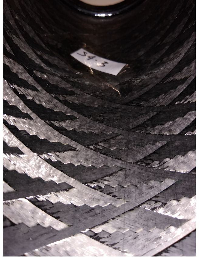
Figure 16: Inner surface of filament-wound cylinder VAFW4-3. The smooth mandrel produces a significantly smoother inner surface on the cylinder compared to the outer surface.
