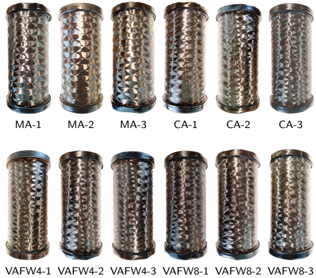
Figure 2: Filament-wound cylinders used in the imperfection measurements. Outer diameter: 136mm; length including resin casting: 300 mm; shell nominal thickness: 0.8 mm; resin casting cross section: 15 × 15 mm.
