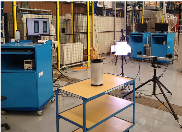
Figure 4: Experimental setup for the DIC measurements.
