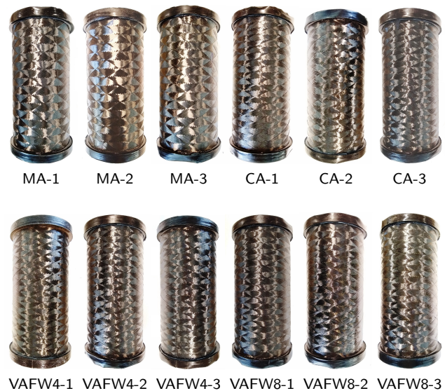
Figure 2: Filament-wound cylinders used in the imperfection measurements.
