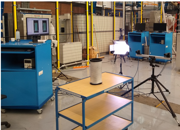
Figure 4: Experimental setup for the DIC measurements.
