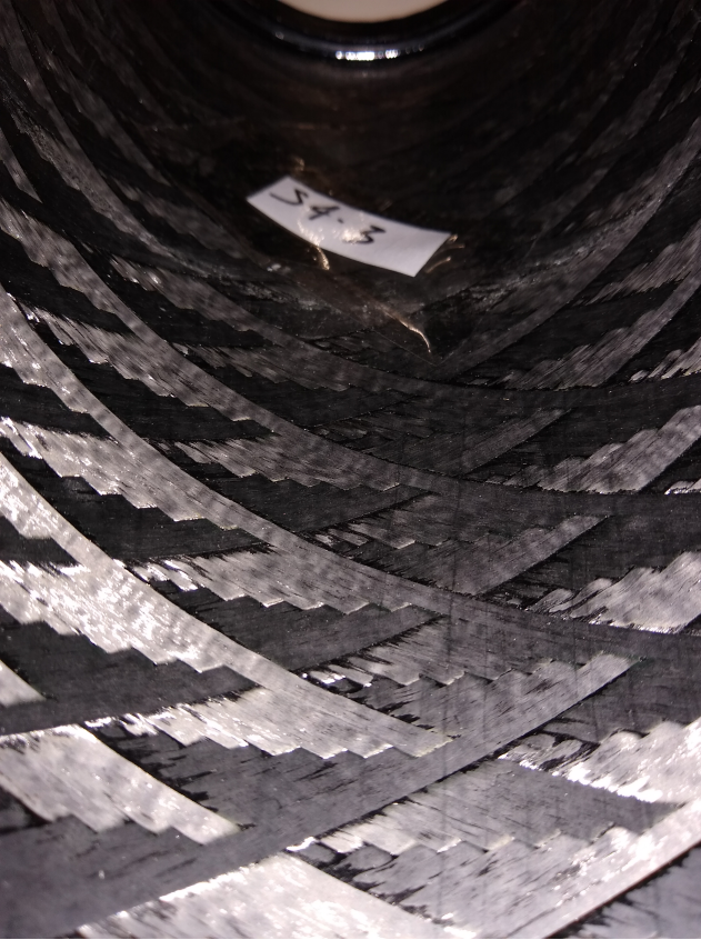
Figure 16: Inner surface of filament-wound cylinder VAFW4-3. The smooth mandrel produces a significantly smoother inner surface on the cylinder compared to the outer surface.
