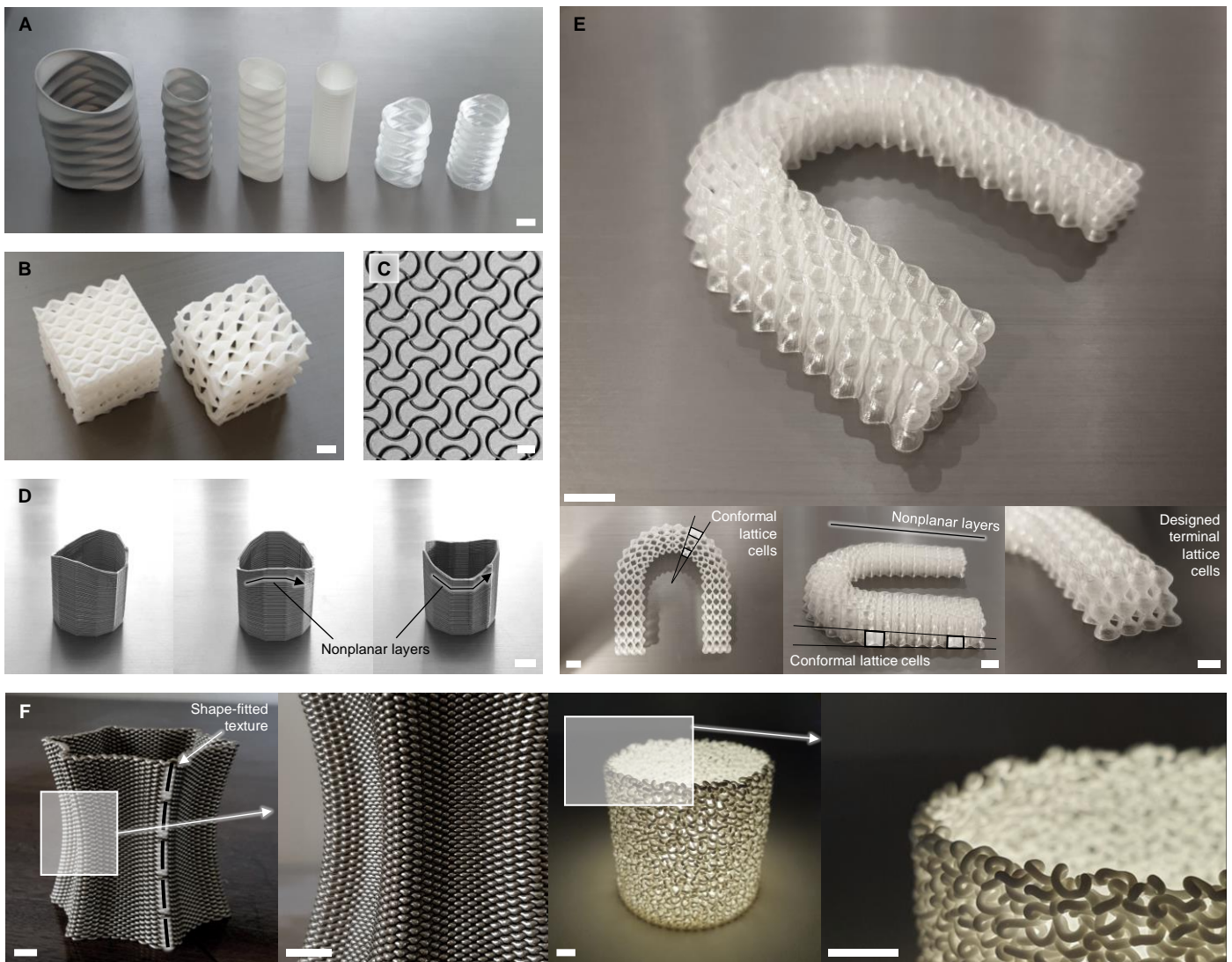
Figure 5 Mathematically defined structures produced using FullControl GCode Designer. A) Parametric spiral print-path with sinusoidal fluctuation, created with a single design feature in FullControl. B) Gyroid lattice structures. C) Lattice structure considered in Figure 3. D) Dodecagonal cylinder with sinusoidally varying layer height designed with just three features in FullControl. E) A concept shoe sole with conformal lattice geometry, nonplanar layers and specially designed terminal lattice cells - designed with just thirteen features in FullControl. F) Mathematically defined textures. Videos S1 and S4 in supporting data [34] show the printing process for (C) and the manufactured part in (E), respectively. Scale bars = 5 mm.
