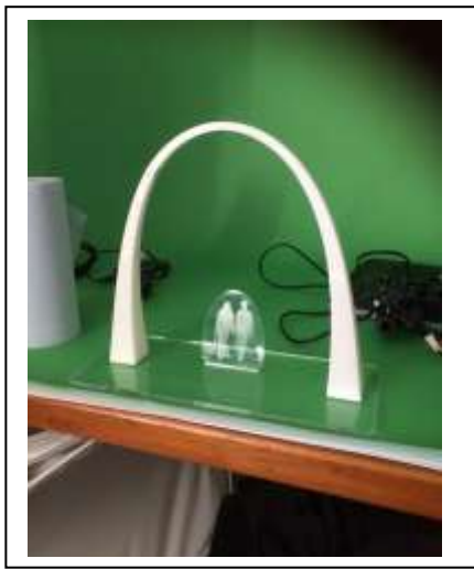
Figure 6 Stand-alone, constant stress arch (a) 1:20 model (b) arch centre-line profile. The model and image in (a) courtesy of M. Millson, University of Warwick
