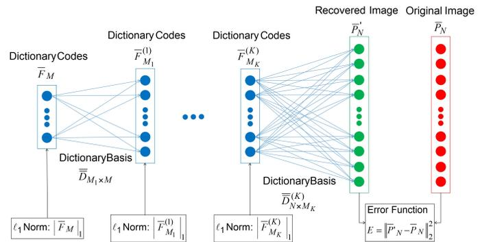
Fig. 3. The working principle of the DLNet to learn the sparse dictionary basis of the face images.
