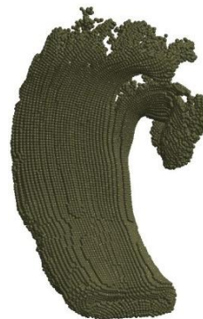
Fig.18c Jacket fragmentation at 0.55ms after exit
