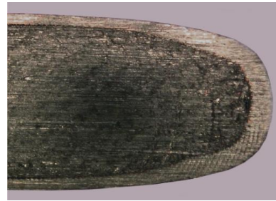
Fig.4b Bullet nose detail: lead core with copper-alloy jacket
