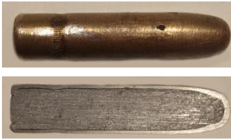
Fig.4a Parravicini-Carcano bullet: mid plane section cut of jacket and lead core
