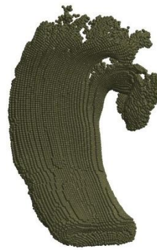
Fig.18c Jacket fragmentation at 0.55ms after exit
