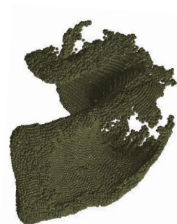
Fig.18d Jacket fragmentation (opposite perspective)
