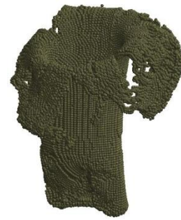
Fig.17d Jacket fragmentation at 0.55 ms after exit
