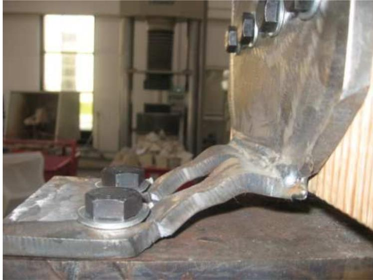
**Figure 18.** Failure of the XL-stub after the variable amplitude cycles test
