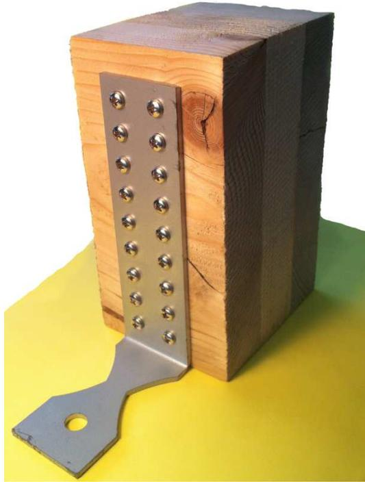
**Figure 6.** Concept of the developed dissipative angle (study model)
