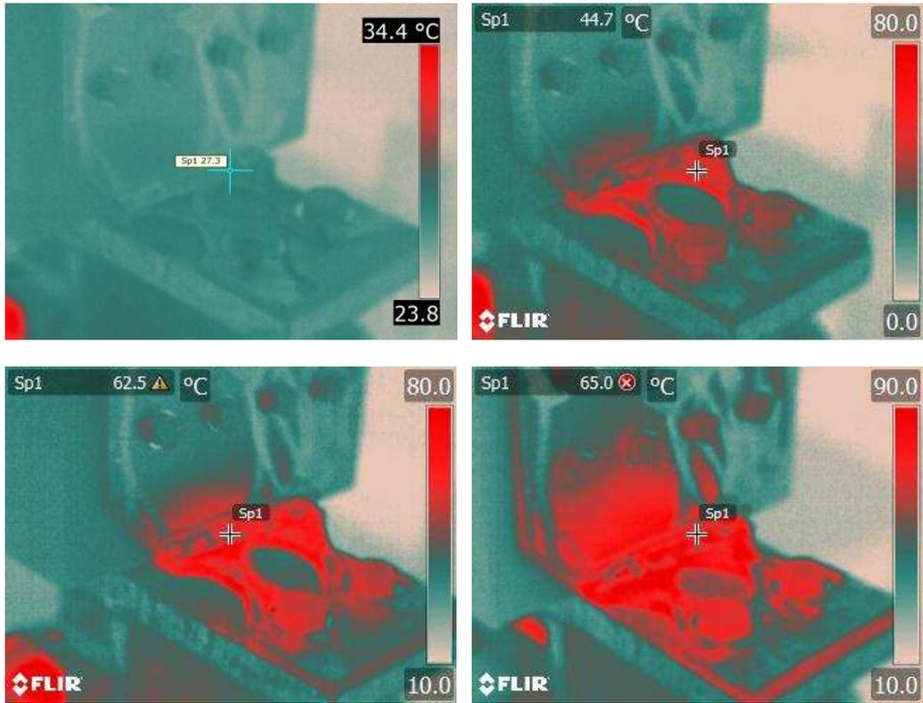
**Figure 15.** Shots took with thermal camera in the first six cycles of loading
