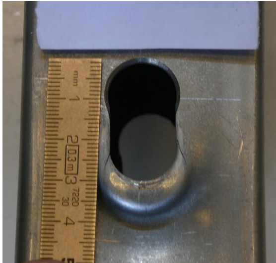
a) Local buckling failure at the bolt hole (Test HX-2-M16)
