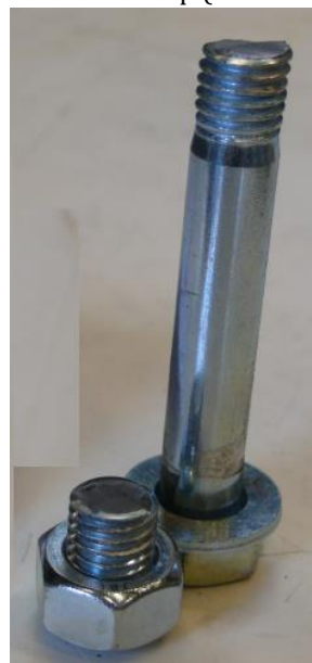
d) Bolt failure (Test S235-4-M12)
