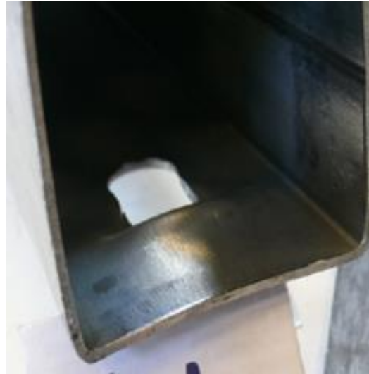
b) Local buckling failure at the bolt hole, particular of the bump (Test HX-2-M16)
