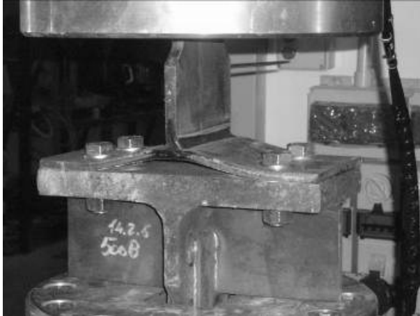
Figure 9: Experimental test on rectangular T-stub on rigid support
