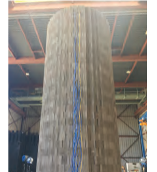
Fig. 4. General layout of physical models at a) Caltech ( \lambda_\ell = 1/107 ), and b) UCB ( \lambda_\ell = 1/25 ). c) Schematic of the experimental layout with the model centered on top of the shake table platen, whose motion is observed by two cameras procuring high-speed photographs in real time, and additional instrumentation consists of laser velocimeters and accelerometers. d) Typical snapshots produced by high-speed photography and digital image correlation. e) Closeup of laser velocimeters and accelerometers. f) Accelerometer array on the back of towers at UCB.
