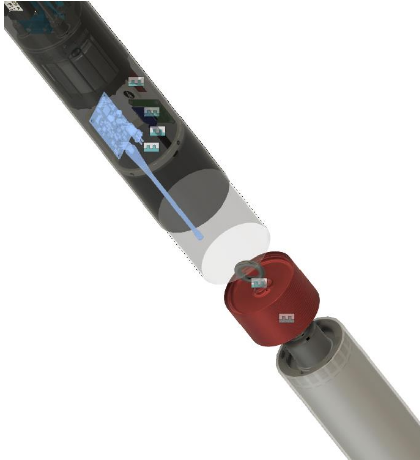
Figure 4.7.5. Exploded diagram of Lumineer's lower avionics bay.
