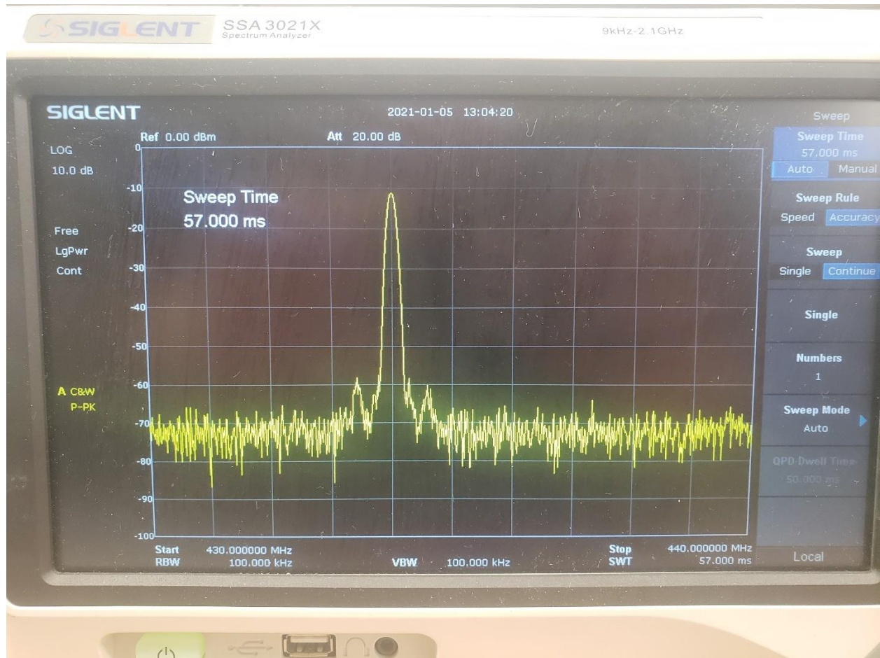
Figure 3.13. Ground station board transmitting an unmodulated sine wave. ~40dBm of attenuation has been applied.
